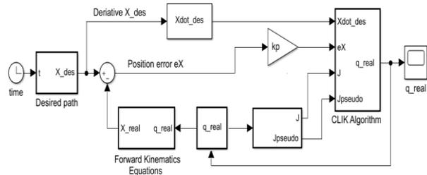
Figure 2. CLF algorithm model implemented in MATLAB/SIMULINK
