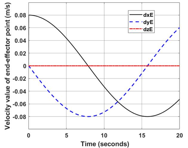
Figure 4. EE point velocity value in the workspace
